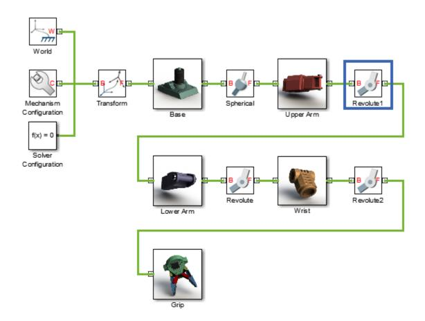
Joint blocks are assortments of joint primitives, basic yet complete joints of various kinds you cannot decompose any further—at least without losing behavior such as the rotational-translational coupling of the lead screw joint. Joint primitives range in number from zero in the Weld Joint block to six in the Bushing Joint block. There are five joint primitives:
